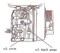
Drain the used oil when the engine is warm. Warm oil drains quickly and completely
