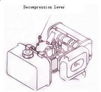
③Start :Hold the starting handle firmly .pull the rope hard and fast .pull it all the way out .use two hands if necessary.
