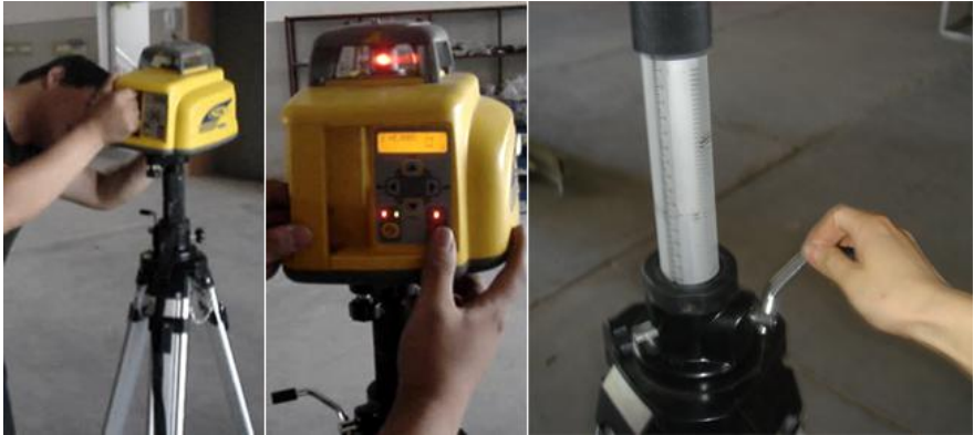
Pic 5.2 Installation of transmitter
