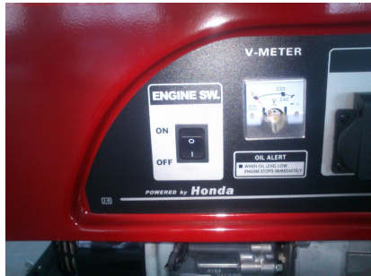
Pic 5.5 stop switch of generators
