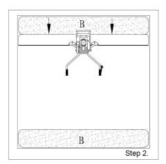
Place one end of the float blade on each of the parallel strips (B) and screed the concrete (C) in between the strips. Be sure the float blade follows the contour of the parallel strips
